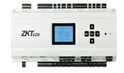
The EC10 Elevator Control Panel can restrict access up to ten floors. Each EC10 can support up to three EX16 boards. When combining together, a total fifty eight (58) floors can be controlled with a single EC10 bundle. Note EC10 panels can be daisy-chained together to control as many floors as desired.
